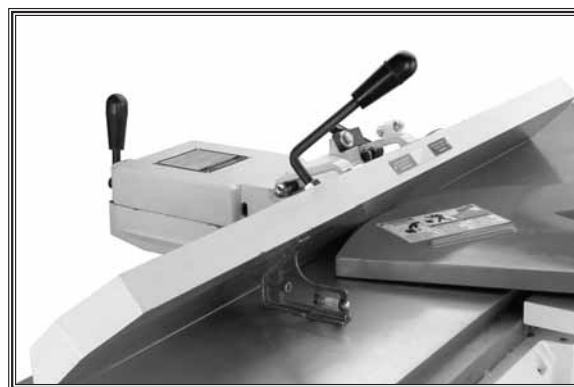
Figure 53. Fence adjusted 45° inward.
