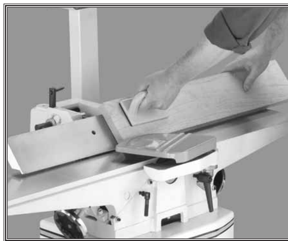
Figure 34. Typical bevel cutting operation.
