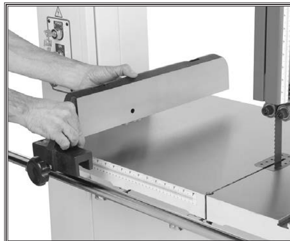
Figure 15. Installing fence onto rail.
