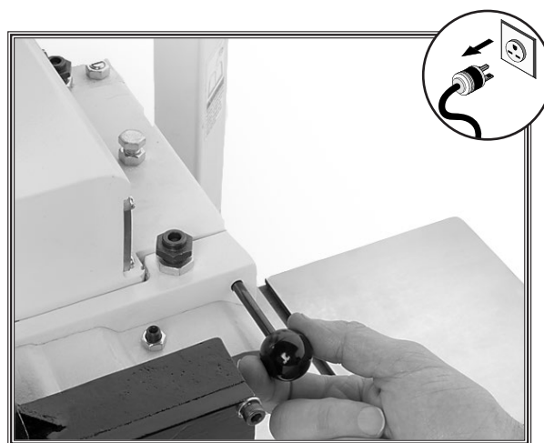
Figure 18. Removing chip deflector retaining pin.
